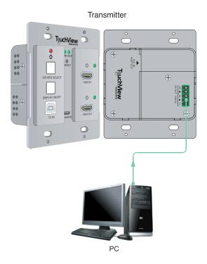
② When control the far-end third party device from local control device (e.g. PC), please connect the PC to the RS232 port of the transmitter, and then please connect the third party device (e.g. projector) to the RS232 port of receiver. The connection diagram shown as below:
