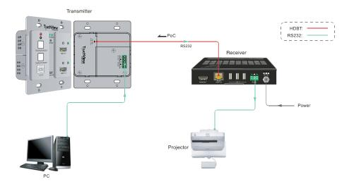
(3) When control the local third party device from far-end control device (e.g. PC), please connect the PC to the RS232 port of the receiver, and then please connect the third party device to the RS232 port of transmitter. The connection diagram shown as below:
